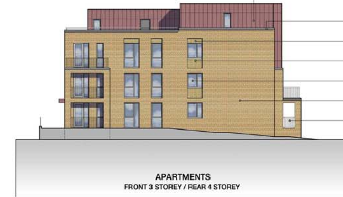
ELEVATION 5 / WEST ELEVATION - BLOCK E
