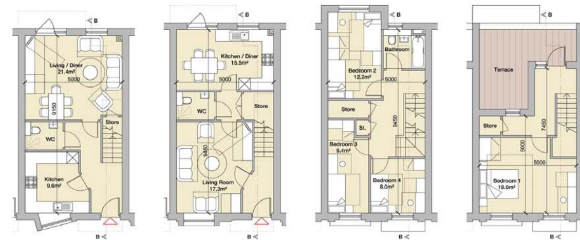
UNIT PLANS - 2no. GROUND FLOOR 4 BED / 6 PERSON TOWNHOUSE @ 122.5m 2 UNIT 21 (AS) / UNIT 38 (HANDED) UNIT PLANS - 6no. GROUND FLOOR 4 BED / 6 PERSON TOWNHOUSE @ 126.5m 2 UNITS 18-20 (AS) / UNITS 39-41 (HANDED) FIRST FLOOR SECOND FLOOR
