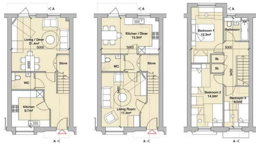
UNIT PLANS - 2no. GROUND FLOOR 3 BED / 5 PERSON TOWNHOUSE @ 98.4m 2 UNIT 15 (AS) / UNIT 44 (HANDED) UNIT PLANS - 4no. GROUND FLOOR 3 BED / 5 PERSON TOWNHOUSE @ 98.4m 2 UNITS 16-17 (AS) / UNITS 42-43 (HANDED) FIRST FLOOR
